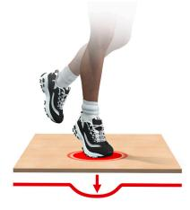
**POINT ELASTIC:** The floor surface deflects only where the foot makes contact with it. This can "trap" the foot and restricts movement Eg. Vinyl, linoleum, P.U. or rubber glued to screed.
